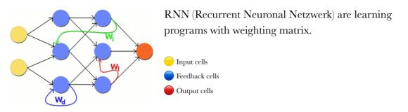
In recurrent neural networks, the neurons of the same layer  $\bigcirc$  or of different layers  $\bigcirc$  are fed back. These feedbacks allow time-coded information to be extracted from data.
